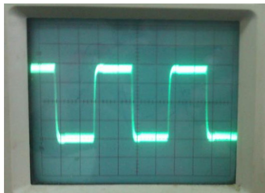
Figure 6 – Waveform of the voltage at the output of the inverter with a capacitor in the primary circuit of the transformer
