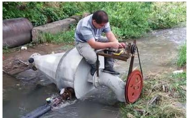
Figure 6 – Types of mini HPP when water is supplied to the hydrocyclone housing through the pipe and partially through the inlet pipe
