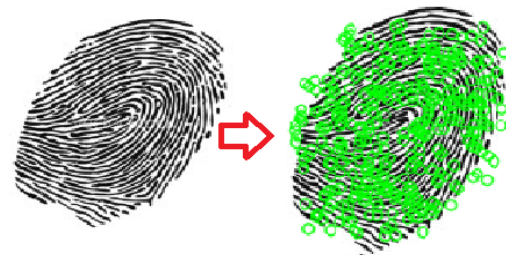
Figure 5 – Evaluation of keypoints of SURF descriptor
