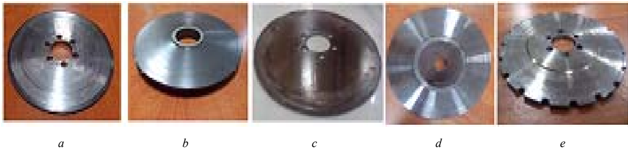
Figure 2 – The photographs of the cutting blades: (a) a cutting blade of steel 65D; (b) a cutting blade of steel 50; (c) a cutting blade of steel 45; (d) a cutting blade of steel Hardox (e) a cutting blade of steel 20
