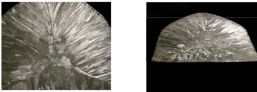
Figure 3 – Macrostructure of an aluminum alloy ingot with the response of the generalized structure of the thermal field
