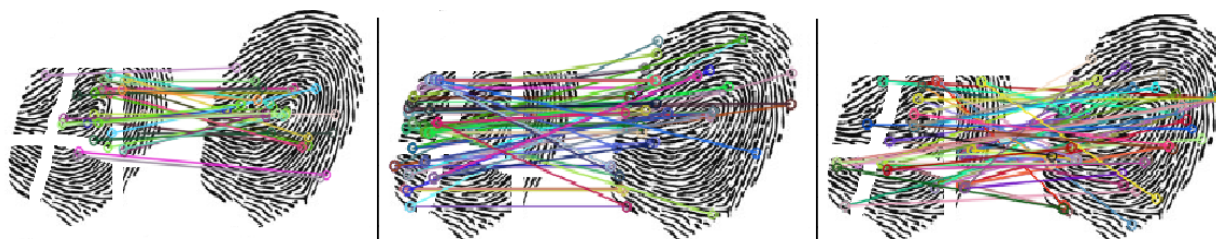
Figure 9 – Score 30 key points descriptor ORB (left), SIFT (center), SURF (right)
